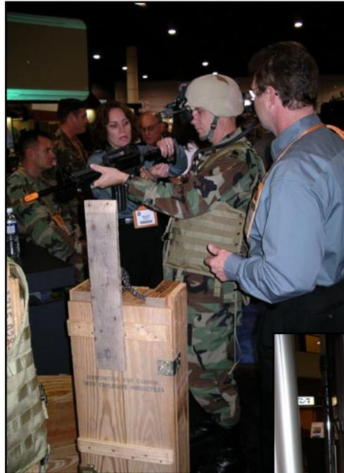
**FIGURE 7.** Samuel Grimes tries on the DAGGERS outfit with the assistance of Quantum3D's Arnold Estep. The box in front of them contains the tracking system. The gun, as well as the soldier's head and body, are all tracked. The Thermite computer and battery pack are hung on the back of the vest. (Photo: Ben Delaney, CyberEdge Information Services)
