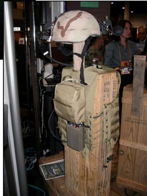
**FIGURE 8.** Here's the Thermite system from the back. The batteries are in the pouch and the computer is mounted below them. (Photo: Ben Delaney, CyberEdge Information Services)
