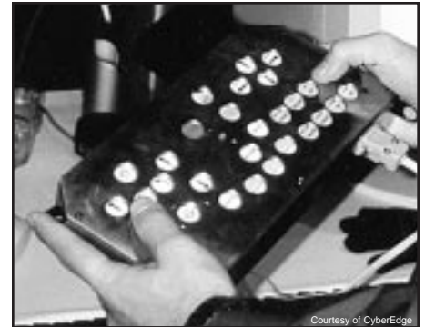
A replica of the control panel used to operate 5DT's Continuous Mining Machine Simulator.
